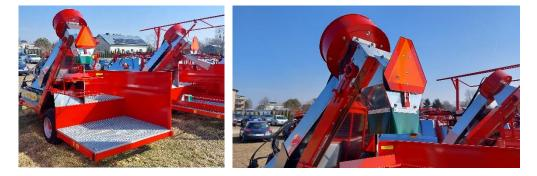
4. Special transport tow bar for three-point hitch
