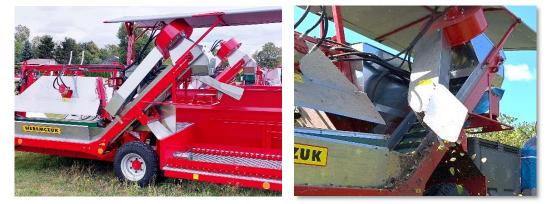
**10.** Complete equipment for high haskap, with divided steel shaking discs (additional shaking with fingers - 5 pcs, special element for lifter, steered exhaust air cover)
