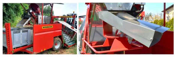
4. Sequential grate for small boxes (alternatively to the two-level grate)
