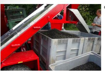
c. The Joanna harvesters **do not require additional transport attachments on wheels** (carts) to collect into the big 500 kg boxes. In addition, our solution provides greater safety of unloading them by the rigid mounting of rollers on the harvester's platform. Furthermore, in order to change a set from standard boxes to big 500 kg boxes or vice versa, only a few operations have to be done requiring one hour of work maximum.
