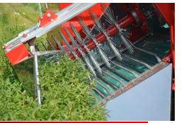
JOANNA 5 CLASSIC JOANNA 5 PREMIUM The harvester has an innovative and patentpending design of row divider that is not used in any other berry harvester. The divider position can be easily adjusted to harvest any height above 35 cm heights and any row width. This solution allows also to harvest fruit from young shrubs in the second year of fruiting.
