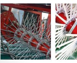
Weremczuk FMR company, due to different customer requirements for the harvest of its own plantation, proposes **two types of "shaking elements".** Some people prefer steel shaking rods because of the speed of harvesting. Customers who have the most delicate shrubs buy modular rods made of special plastic.
