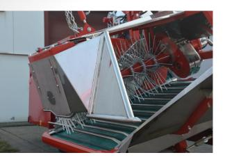
Joanna harvesters are equipped with a complete set of covers made of stainless steel. The use of stainless steel in Joanna machines guarantees their durability and keeps the machine clean for many years. Let us remember that crops reaching up to 2.5 meters in height during harvesting have a huge impact on covers and machine collecting components. Therefore, tarpaulins and plastic covers used by competitors do not provide suitable strength and reliability to work for many years.
