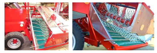
3. Special element for lifter (bringing the lifter`s beak closer to the row) recommended for haskap and gooseberries
