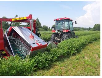
Harvesting with machines of berry bushes under 35 centimeters high (regardless of the machine brand) can cause damage to plants - disrupting their following growth or increasing the risk of disease. Out of concern for good yields to our customers, Weremczuk FMR recommends a mechanical harvest of bushes from 35 centimeters and above. Therefore, marketing advertisements of competing producers with the possibility of harvesting from 20 centimeters may expose customers to serious losses in crops.
