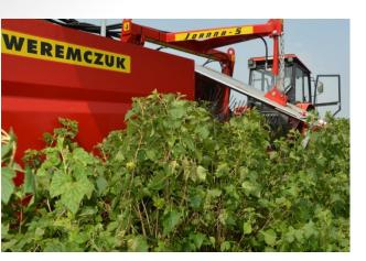
All JOANNA harvesters are based on a **shaking unit with one shaker equipped with a special, patented** (Patent No. 219881, competition does not have patents) **head** that has **6 independent levels of amplitude.** Amplitude control allows us to adjust the harvest strength to each type of berry fruit. In addition, maintenance-free toothed belts are used in the head to drive the head elements (instead of toothed wheels used in other combines), it ensures quiet and trouble-free operation.
