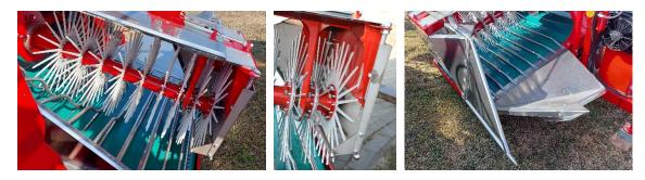
2. Inclined shaker grate cooperating with the inclined position of the shaker
